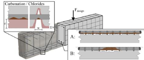
**Task:** This master thesis should contribute to the overall project goal by numerically investigating the fracture behaviour of reinforced steel beams under consideration of degradation processes. Furthermore, the computational model should be embedded in existing safety concepts for nonlinear FE-Analysis (NLFEA):
