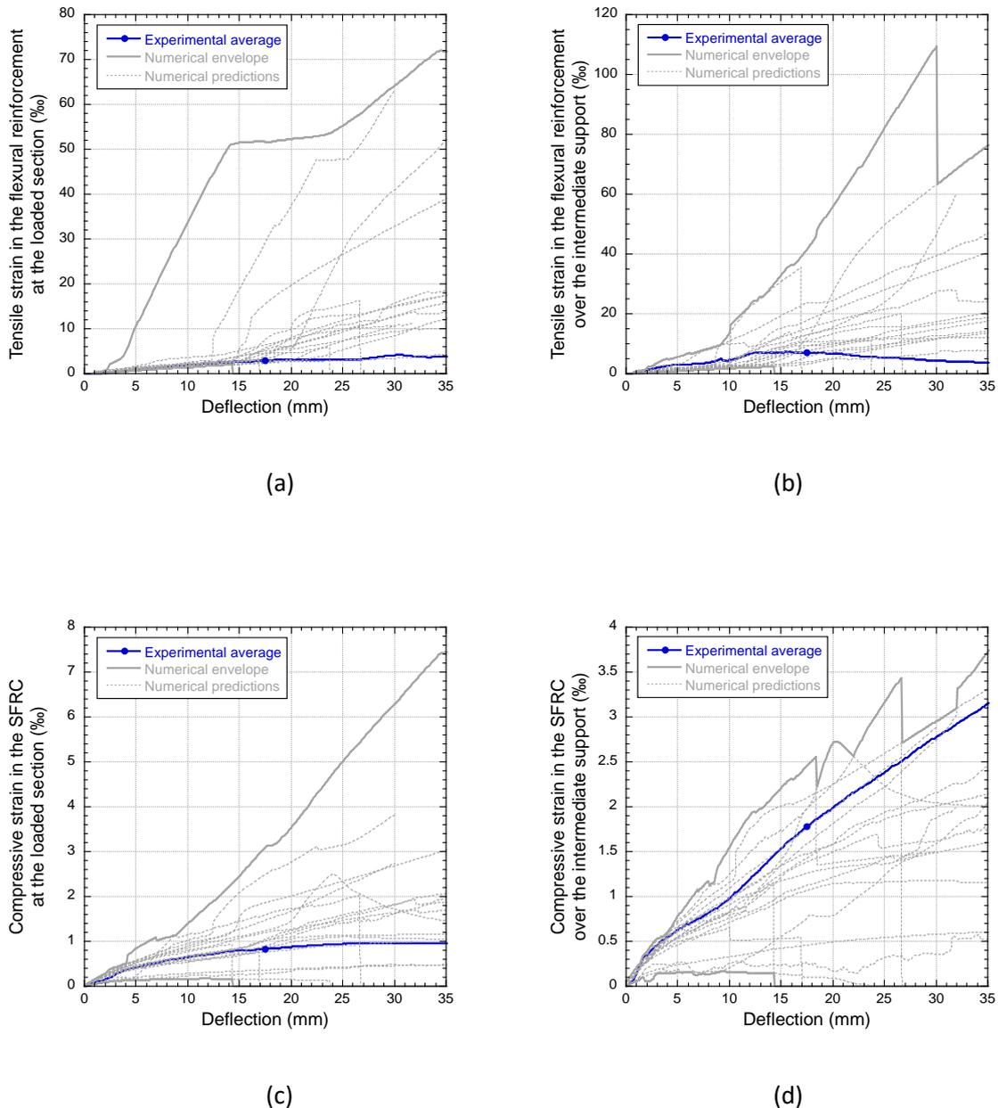
Figure 3. Experimental results, numerical envelope and numerical predictions of all participants regarding the: tensile strain in the flexural reinforcement at the loaded section versus deflection (a), tensile strain in the flexural reinforcement over the intermediate support versus deflection (b), compressive strain in the SFRC at the loaded section versus deflection (c) and compressive strain in the SFRC over the intermediate support versus deflection (d)
