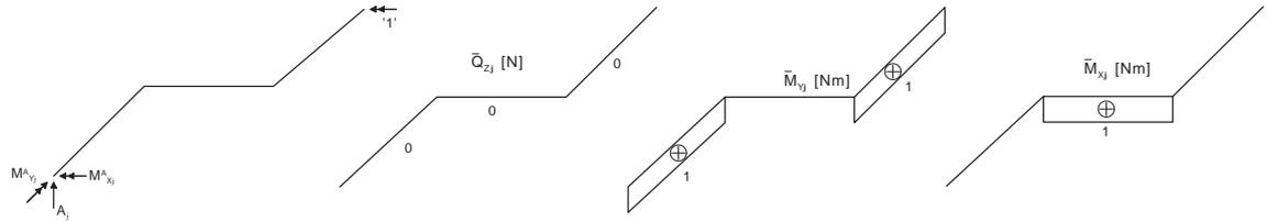
$$\begin{aligned} \bar{A}_\varphi &= 0 \quad N \\ \bar{M}_{X\varphi}^A &= 1 \quad Nm \\ \bar{A}_{Y\varphi}^A &= 0 \quad Nm \end{aligned}$$
