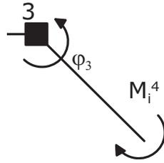
$$\begin{aligned} \rightarrow M_k^2 + M_i^4 &= 0 \\ \Leftrightarrow M_k^{20} + k_{ik}^2 \cdot [2\varphi_3 + \varphi_2] + k_{ik}^4 \cdot 2\varphi_3 &= 0 \\ \Leftrightarrow -1,67 + [2000]\varphi_2 + [6400]\varphi_3 &= 0 \end{aligned}$$
