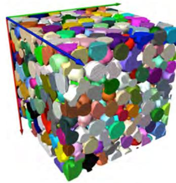
Fig. 3:  $\mu$ CT scan shows a particle distribution of a well-graded granular medium.
