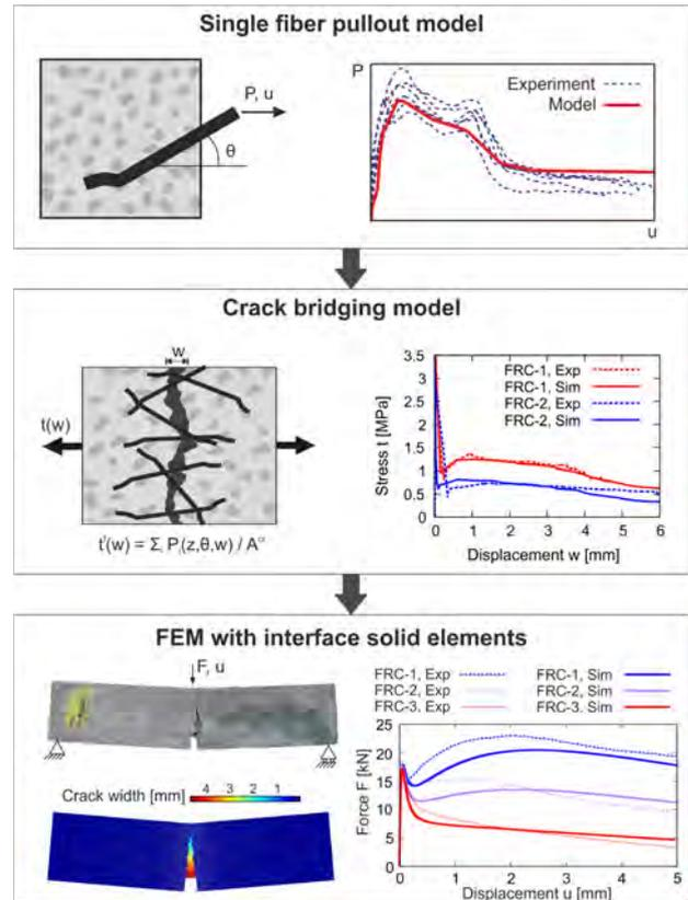
Fig. 3: Modeling of steel fiber reinforced concrete at different length scales.
