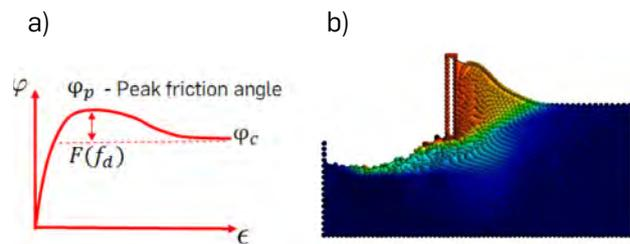
Fig. 6: (a) Control of the peak friction angle value by the model parameter  $f_d$ , (b) Particle Finite Element simulation of soil excavated by a moving tool (colors indicate the particle velocity).
