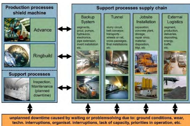
Fig. 1: Interaction of production and support processes in mechanized tunneling.
