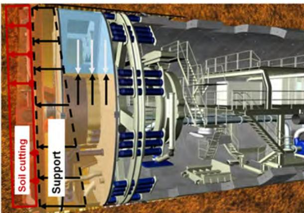
Fig. 1: Hydro shield tunneling (Source: Herrenknecht AG).
