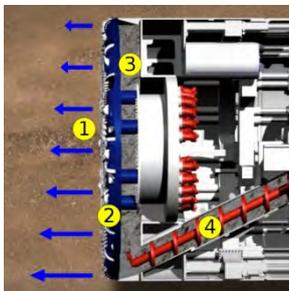
Fig. 1: Aspects of investigation of soil-machine interactions in earth pressure balance tunnel boring machines: (1) face pressure, (2) excavation process and abrasion of cutting tools, (3/4) material flow inside the pressure chamber.
