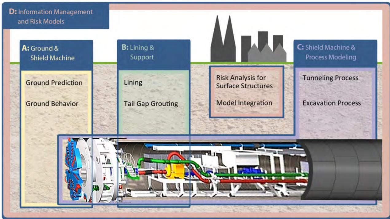
Fig. 1: Components and processes involved in mechanized tunneling and their representation within 4 project areas in the SFB 837.
