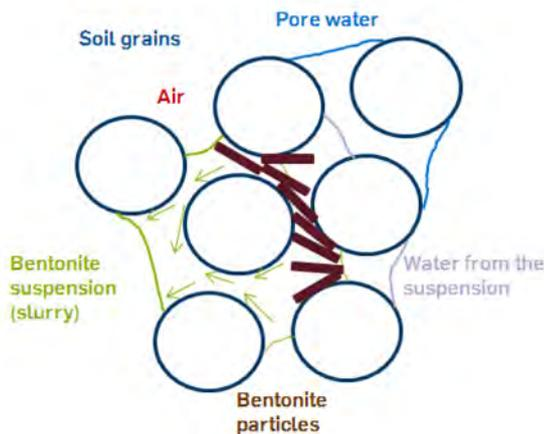
Fig. 4: Changes in soil-system composition.
