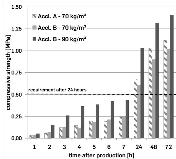
Fig. 3: Compressive strength development up to 72 hours after production with two different accelerators.
