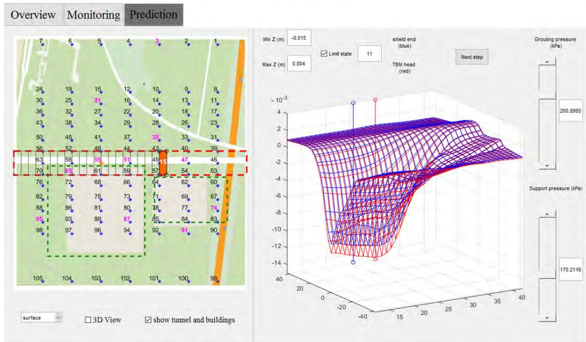
Fig. 3: Simulation and Monitoring-based Assistant for Real-time steering in mechanized Tunneling (SMART).
