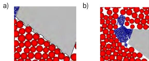
Fig. 2: (a) Failure of the ductile part of the tool (grey), (b) Failure of the brittle tool-part (blue).
