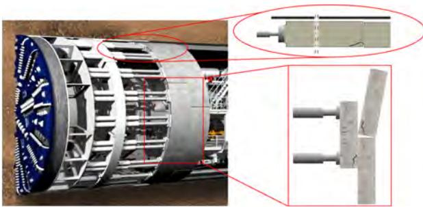
Fig. 1: Possible damage patterns in tunnel lining segments during the excavation process.
