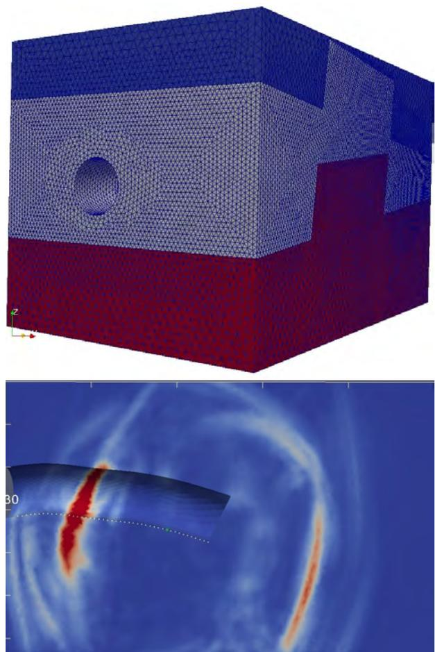
Fig. 1: Top: Tetrahedral mesh with curved tunnel, layer boundaries and steeply dipping faults perpendicular to the tunnel axis. Bottom: Snapshot of the seismic wave field generated by a source at the tunnel face.
