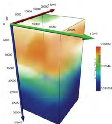
Fig. 2: Porosity distribution as a result of  $\mu$ CT scans of a granular mixture.
