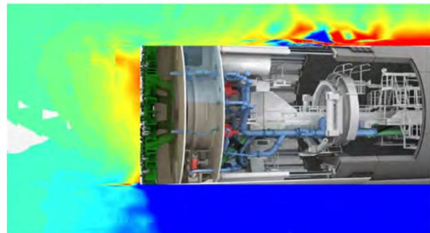
Fig. 2: Excess pore pressure generation around the tunnel.
