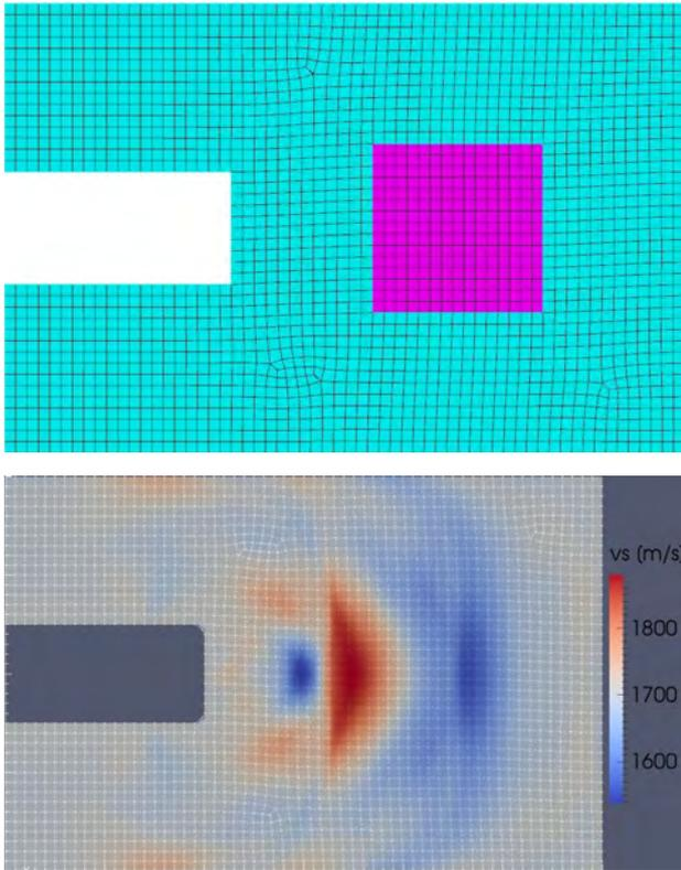
Fig. 2: Simplified test case for the 2D inverse problem in the time domain based on the elastic wave equation. Top: Sketch of the location of a square-shaped structural anomaly in front of the tunnel face. Elastic wave fields were calculated at receivers on the tunnel sidewalls generated by three sources located on the tunnel face. Bottom: Reconstruction of the anomaly using a full-waveform inversion of waveforms recorded at the receivers.
