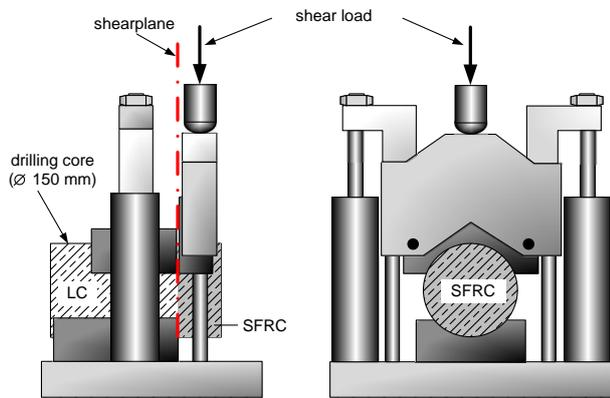
Fig. 2: Test set-up for the shearing test on drilling cores taken from hybrid concrete elements.
