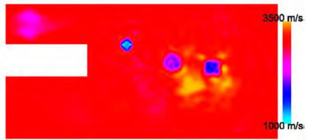
Fig. 3b: Simplified test case for the 2D inverse problem in the frequency domain based on the acoustic wave equation: Reconstruction of the structural anomaly by inversion of spectral amplitudes and phases up to 478 Hz recorded by 33 sensors on the tunnel face and generated by 3 sources.
