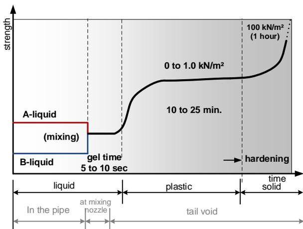
Fig. 2: Strength characteristics of a two-component mortar (TAC Corporation).
