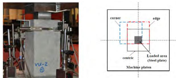
Fig. 1: Test set-up for partial-area loading tests (left) and positioning of the specimen for centric and eccentric loading (right).
