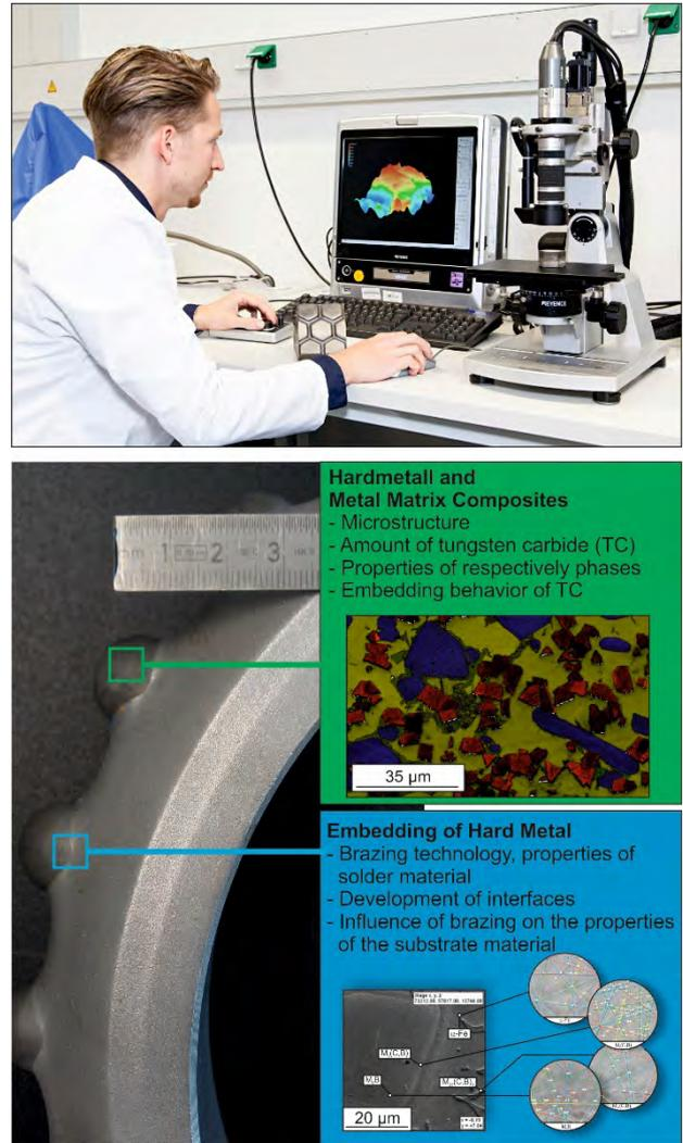
Fig. 2: Investigation of the dominating wear mechanisms of worn tunneling tools using optical and scanning electron microscopy.
