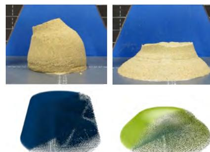
Fig. 1: Slump test – Experiment and simulation.
