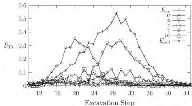
Fig. 2: Sensitivity analysis of decisive subsoil parameters for tunnel driving.
