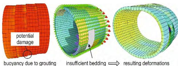
Fig 3: Numerical deformations and Mises stresses for exemplified load case scenario (buoyancy in grouting, insufficient bedding conditions).
