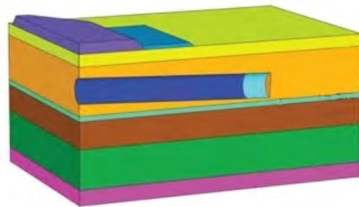
Fig. 1: Numerical Model of the Westerscheldetunnels.
