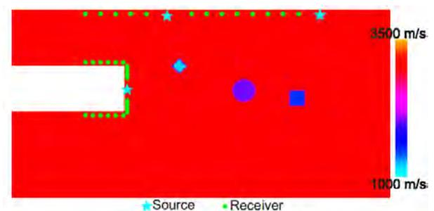
Fig. 3a: Blind test for the 2D inverse problem in the frequency domain based on the acoustic wave equation: Homogeneous test model with embedded structural anomalies.
