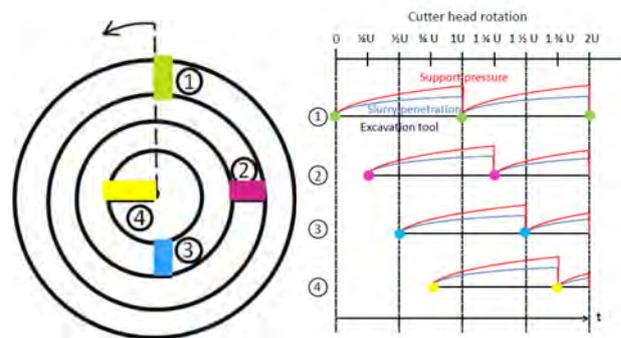
Fig. 2: Arrangement of the cutting tools on the cutter head (left), Superposition of slurry penetration and soil excavation processes (right).
