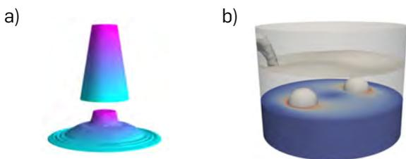
Fig. 5: Numerical simulations for material identification and mixing validation: (a) Slump test, (b) Mixing tank.
