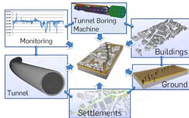
Fig. 1: The tunnel information model consisting of four main sub-models, the time dependent settlements and machine data monitoring.
