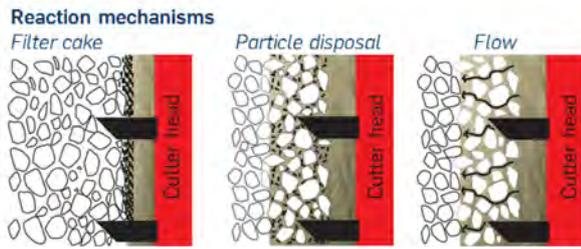
Fig. 3: Reaction mechanisms in the soil.
