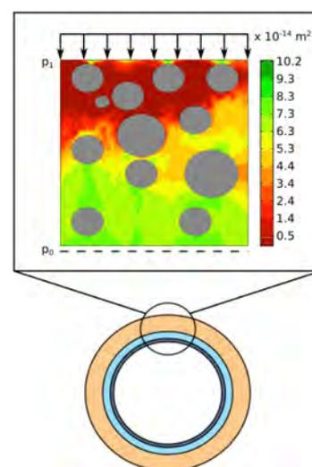
Fig. 1: 1: Permeability distribution in the annular gap and the surrounding soil.
