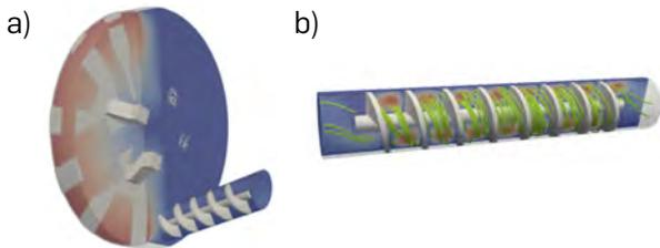
Fig. 4: (a) Simulation of (nearly) realistic EPB geometry with cutting wheel, rotating arms and screw conveyor, (b) Computed streamlines in the screw conveyor.
