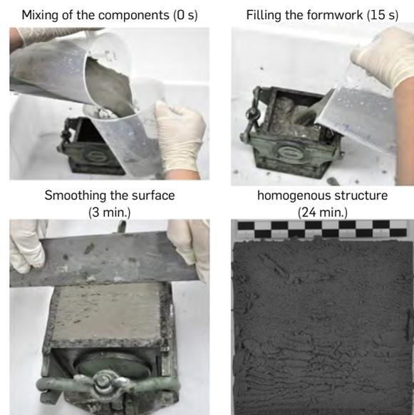
Fig. 1: Sample production of two-component mortar (cube formwork: 100 x 100 x 100 mm<sup>3</sup>).
