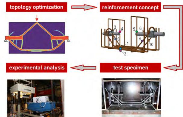
Fig. 4: Steps of the concept for an optimized design for the example of shear coupling.
