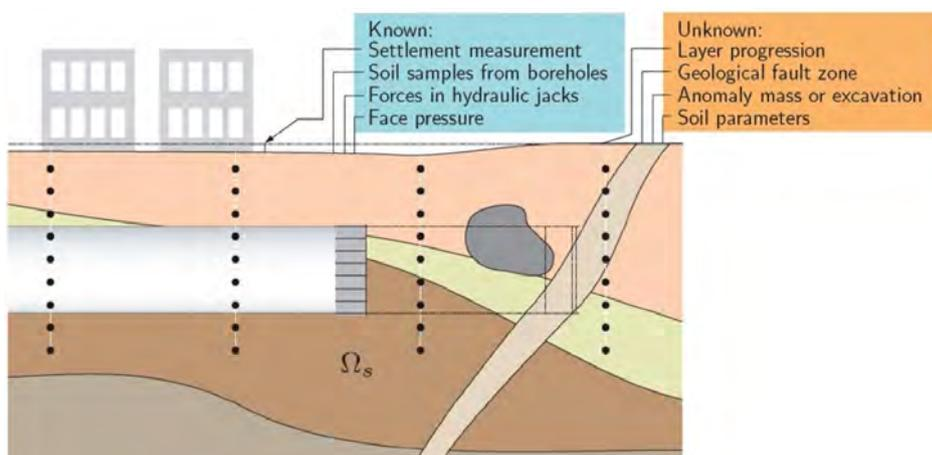
Fig. 4: Identification, validation and adaption of subsoil models based on measurement data.
