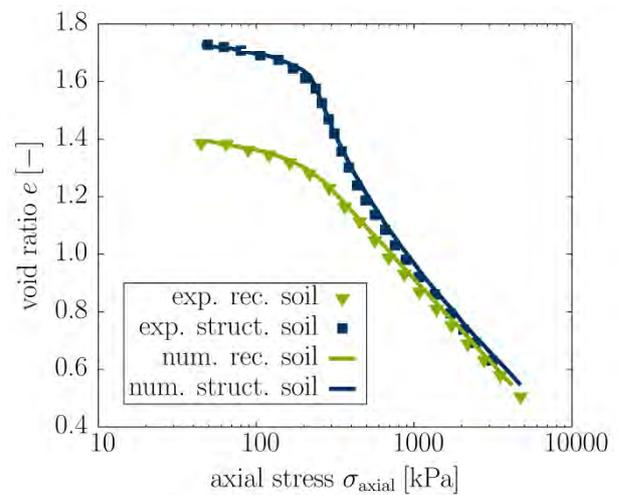
Fig. 4: Compression behavior of structured and reconstituted soil in oedometer tests. Comparison of experimental (symbols) and numerical (lines) results.
