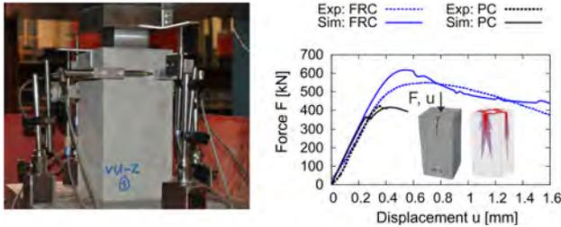
Fig. 4: Partial area loading tests on plain and fiber reinforced concrete. Left: experimental setup. Right: comparison of the force-displacement curves and crack patterns from experiment and numerical simulation for fiber reinforced concrete (FRC) and plain concrete (PC).
