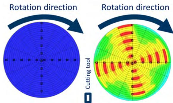
Fig. 5: Model of the homogeneous support pressure transfer (left) and of the transient support pressure transfer (right).
