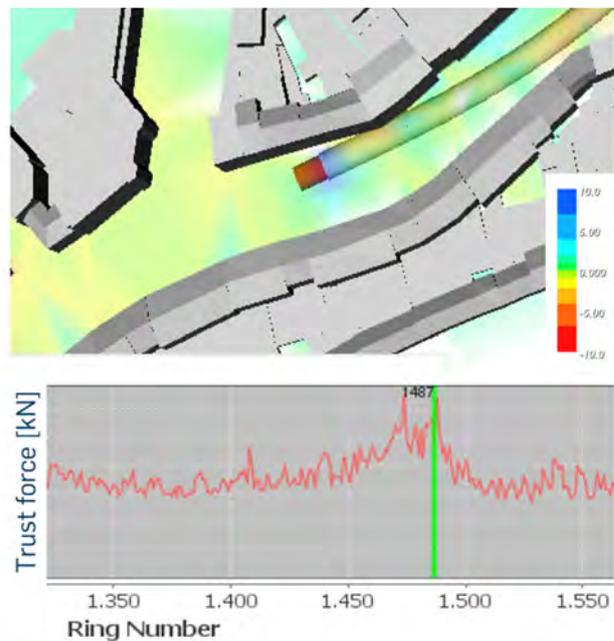
Fig. 3: A visual representation of the connection between settlements and TBM driving forces.
