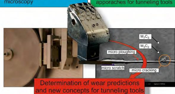
Fig. 3: Performing tribological tests and development of a new wear test to evaluate the residual service life of tunneling tools.
