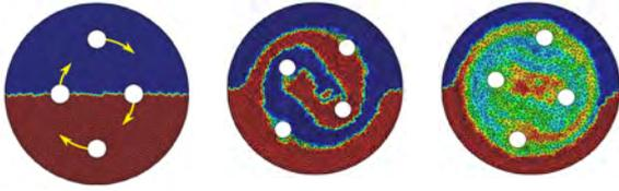
Fig. 3: Mixing process of a viscous two-phase mixture: Evolution of the volume fraction of one phase.
