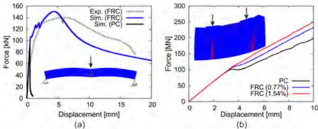
Fig. 5: Numerical simulation of lining segments made of FRC: (a) Ductile behavior under flexural loading; (b) parametric study of the influence of fiber content on the nonlinear responses under thrust forces.
