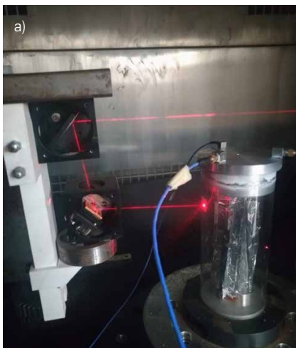
Figure 1: Polymeric circular cylindrical shell with a top mass: a) empty shell; b) water filled; c) filled with non-Newtonian fluid
